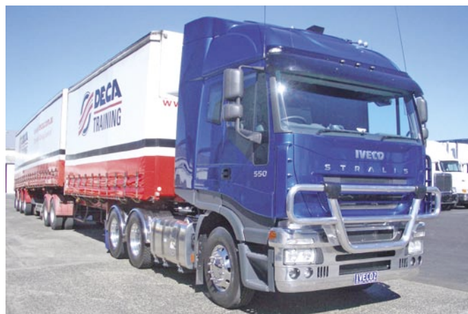
Example of a complying 26 metre B-Double — Cab Strength, Front Underrun Protection, compatible bullbar and 20.6 m trailer set.
