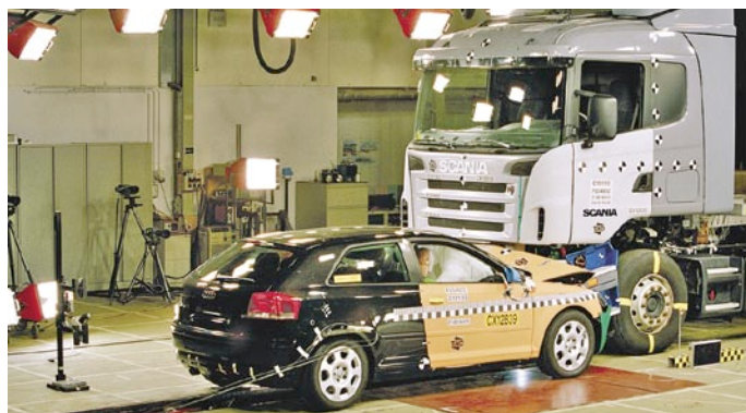
Truck collision Testing of Front Underrun Protection
