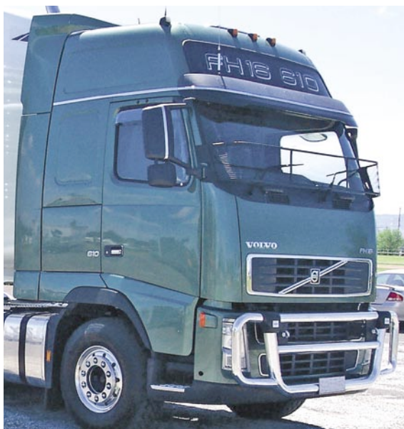
Example of a bullbar that does not interfere with the performance of the FUPS
